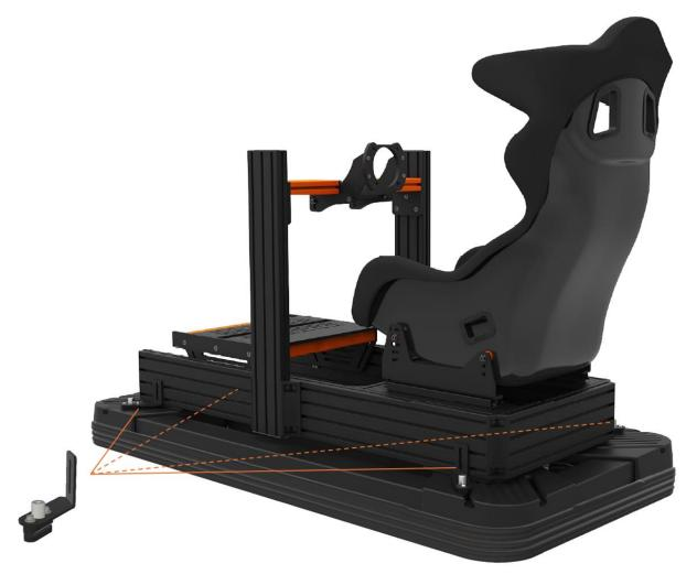
**STEP 4:** Secure all four (4) brackets to the aluminum side profiles using screws and T-nuts (**not included**). Ensure that everything is tight and stable:
