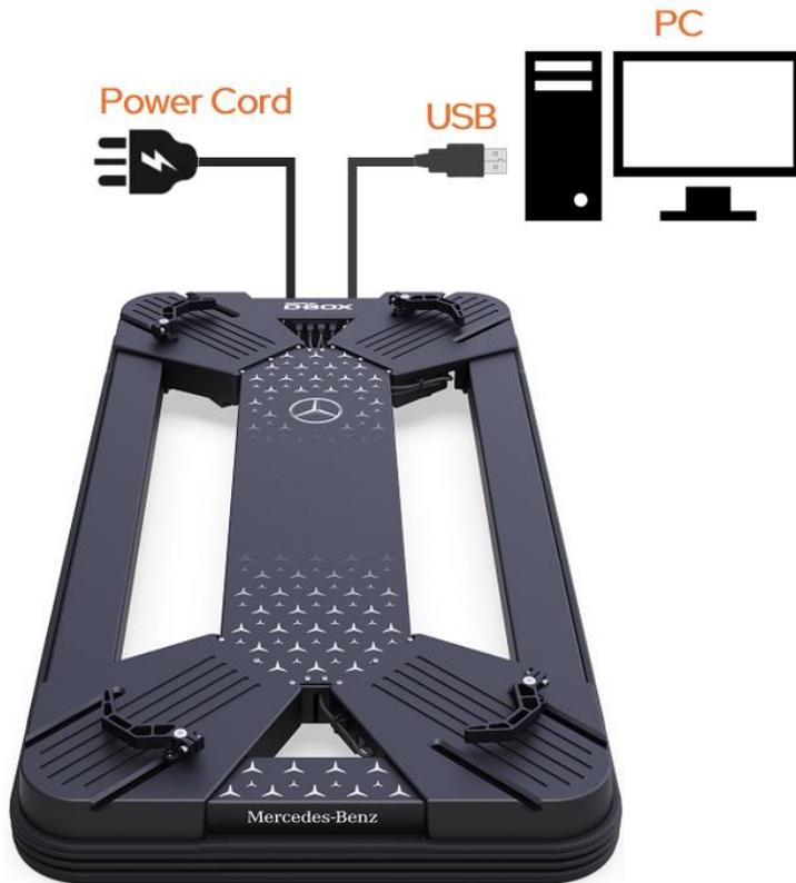
**STEP 1:** Connect the platform to the PC using the provided USB-A to USB-B cable. If needed, you can use the included USB extension to facilitate the connection.
