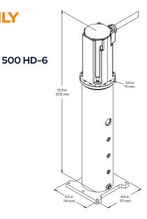
\*HD refers to an actuator designed with a double nut ball screw for higher durability in high strain environment and extended periods of time.
